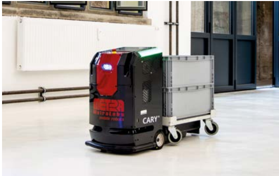
CARY is an autonomous mini-stacker who transports loaded floor rollers.
