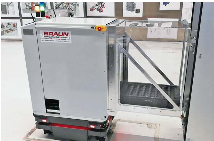
All sensors in the autonomous mobile robot come from SICK.
