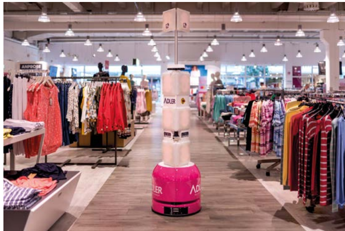
Autonomous robot TORY finds its way between racks of clothes in a clothing store all on its own.
