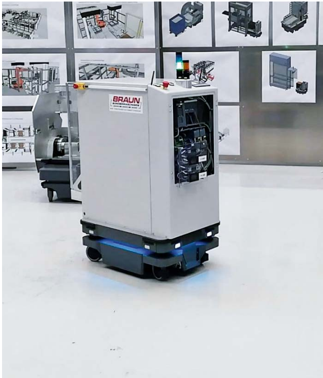
The BS Trayshuttle autonomously picks up small load carriers or trays from one pallet handling machine and puts them down in another pallet handling machine.
