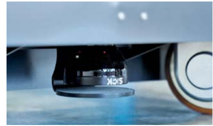
For localization and navigation purposes, three microScan3 safety laser scanners are installed under the vehicle floor.
