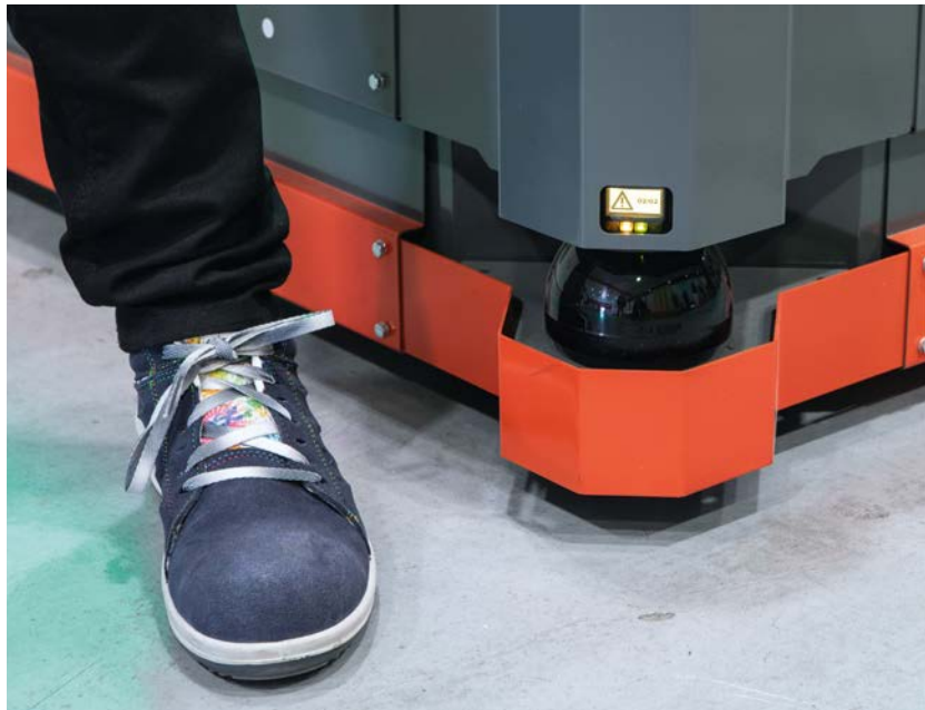
Safety laser scanner microScan3 ensures optimal and safe operations of the AMRs and proves high resistance to dirt, dust, and the incidence of sunlight thanks to the innovative safeHDDM® scanning technology.
